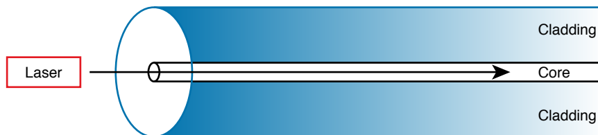
Figure 2-17 Transmission on Single-Mode Fiber with Laser Transmitter
