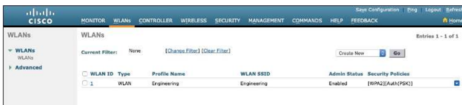
Figure 29-20 Displaying WLANs Configured on a Controller
